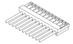
This connector is for wire to board connection with 1.0 mm pitch insulation displacement connection, which achieved miniaturization with mounting height 20 mm and depth 45mm. The twin U-slots and the -point grip construction provides excellent connection performance.
